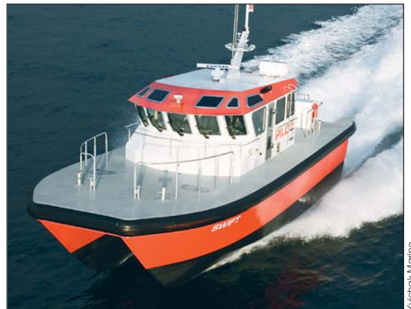
Virginia pilot boat features a foil-assisted design.
